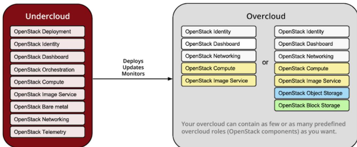
The overcloud underlay consists of three OpenStack controllers, which host the OpenStack services. These are deployed on three bare metal servers. Each set of controllers are deployed in a high-availability (HA) fashion using pacemaker, running quorum, and deployed under the default Keystone version 3 domain. The controllers are deployed using heavily
