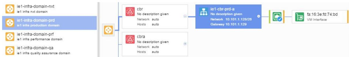
When delivery teams on-board to i2 they are allocated two /26 network subnets per environment. This allows them to deploy A/B immutable subnets, with each release tied to a unique subnet that alternates. When a release is complete, the previous VM's and subnets and ACL rules are automatically cleaned down. This keeps the environment clean over time.
