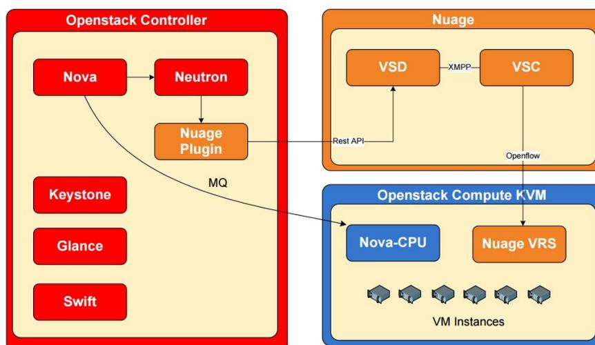
When a Neutron command is issued to OpenStack, the Nuage plugin uses REST calls to communicate with the Nuage VSD and vice-versa. This then communicates with the VSC using XMPP (<https://xmpp.org/>).
