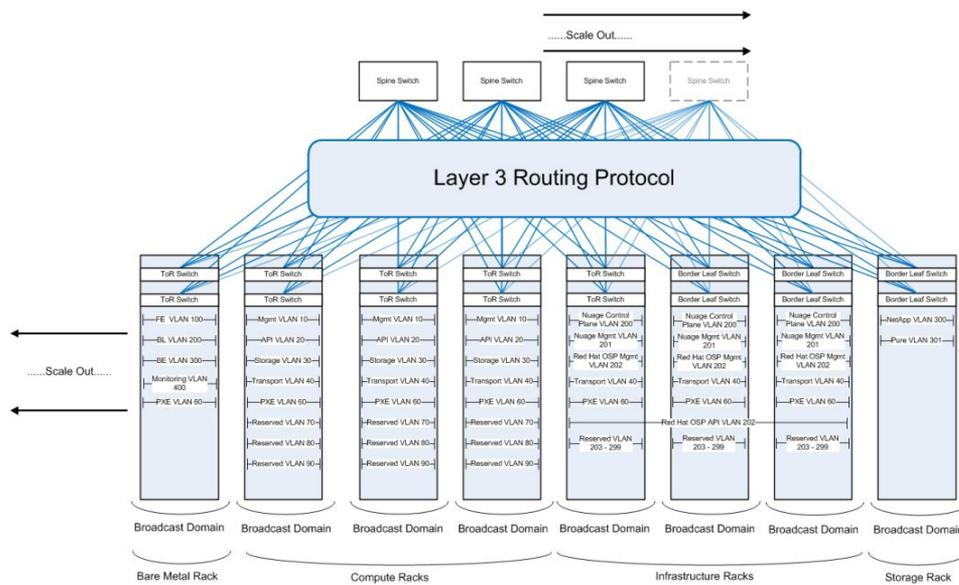
Arista switches are updated using Arista ZTP (Zero Touch Provisioning) once they are racked and cabled in the data center. These pull configuration from the Arista's CloudVision Exchange (CVX) platform which contains all routing information for the Arista switches. Arista's CVX platform provides single point abstraction of the physical infrastructure to the Nuage SDN controller.
