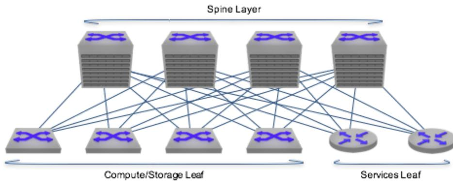
The data center infrastructure is based on the following principles and uses Arista to create the leaf-spine architecture. This gives the ability to scale out by simply adding further racks.
