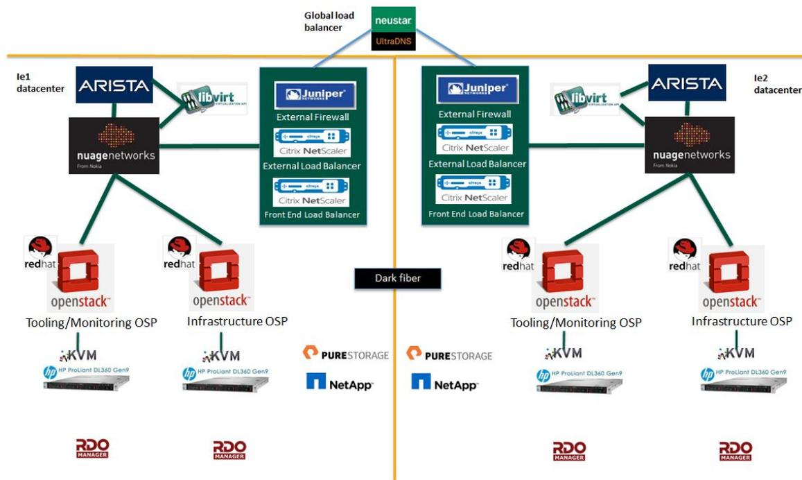
Paddy Power Betfair runs an active-active data center configuration. This utilises UltraDNS to route traffic through an external Juniper firewall to two tiers of Netscalers. Tier 1 (External Load balancing) is used for SSL offload, while Tier 2 (Front End Load Balancing) is used to route traffic to the various applications. This design is mirrored across both data centers.
